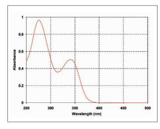
Tinuvin 1577 exhibits strong absorbance in the 300-400 nm region and minimal absorbance in the visible region (>400 nm) of the spectrum. The absorption maxima are at 274 nm and 341 nm ( $\varepsilon$  = 22'000 l/ mol·cm) in chloroform solution.
