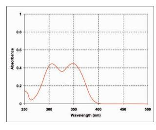
Tinuvin 571 exhibits strong absorbance in the 300–400 nm region and minimal absorbance in the visible region (>400 nm) of the spectrum. The absorption maxima are at 303 nm and 343 nm ( $\varepsilon$  = 14'210 l/mol·cm) in chloroform solution.
