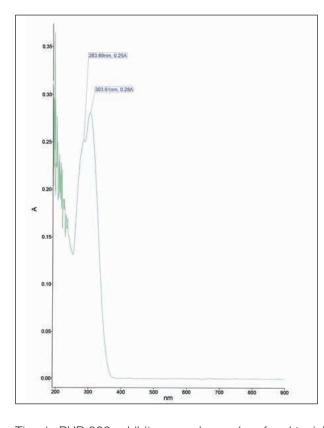
Tinuvin PUR 866 exhibits high absorbance in the 300-400 nm region and minimal absorbance in the visible region (> 400 nm) of the spectrum. The absorption maxima are at 306 nm and 347 nm ( $\varepsilon$  =14760 l/mol·cm) in chloroform solution.
